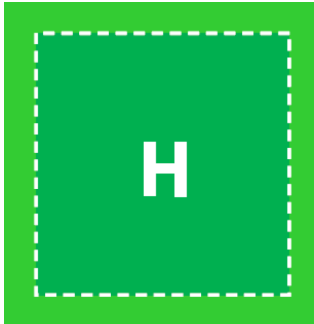
Figure 1: A 1.5 \times D FATO with additional 0.25 \times D Safety Area (Total area is 2 \times D ). Also showing 'H', FATO perimeter and 0.5 \times D Touchdown/Positioning Markings (TD/PM).
